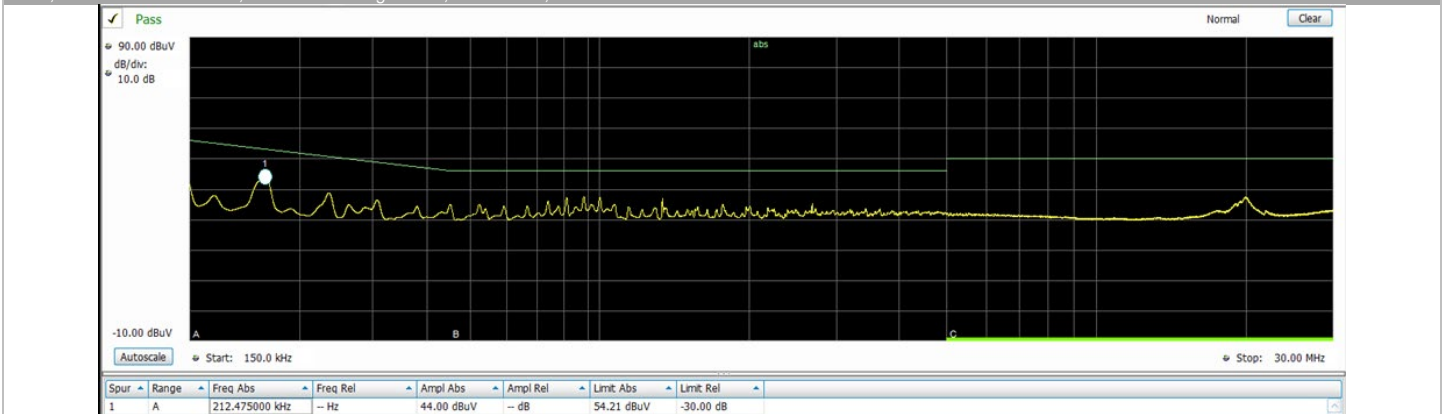
EMI; Conducted CISPR 22; Peak vs. Average Limit; L2/Neutral; 208Vac 24Vdc @ 25A
