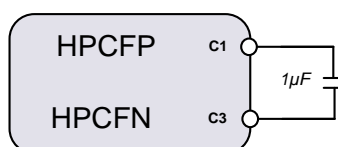
Figure 41: Charge Pump Flying Capacitor
