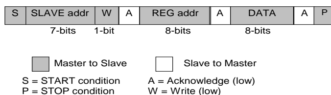
Figure 27: I 2 C Byte Write (SDA signal)
