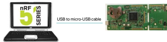
Figure 12 Configuration for application development with nRF52 SDK
