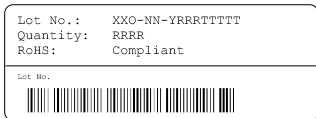
Figure 14: First label on reel: XX = Sensor Type (21 for SHT21), O = Output mode (D = Digital, P = PWM, S = SDM), NN = product revision no., Y = last digit of year, RRR = number of sensors on reel divided by 10 (200 for 2000 units), TTTTT = Traceability Code.
