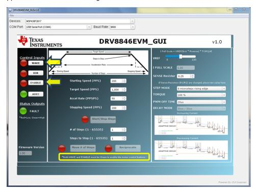
8. The DRV8846 EVM is now awake and can be commanded to turn the motor. This can be done by either selecting the *Start/Stop Steps*, *Move # of Steps*, or *Reciprocate* buttons.
