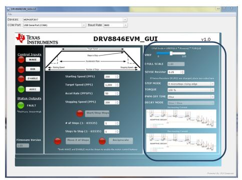
The current is calculated using the VREF slider, the Sense resistor value, the Torque setting, and the Step mode setting using the formula.
