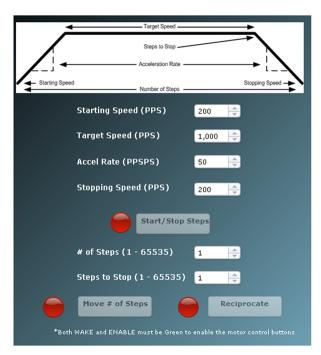
Motor motion can only happen by using an acceleration profile which will be detailed later on. A detailed explanation of each stepper control section follows.
