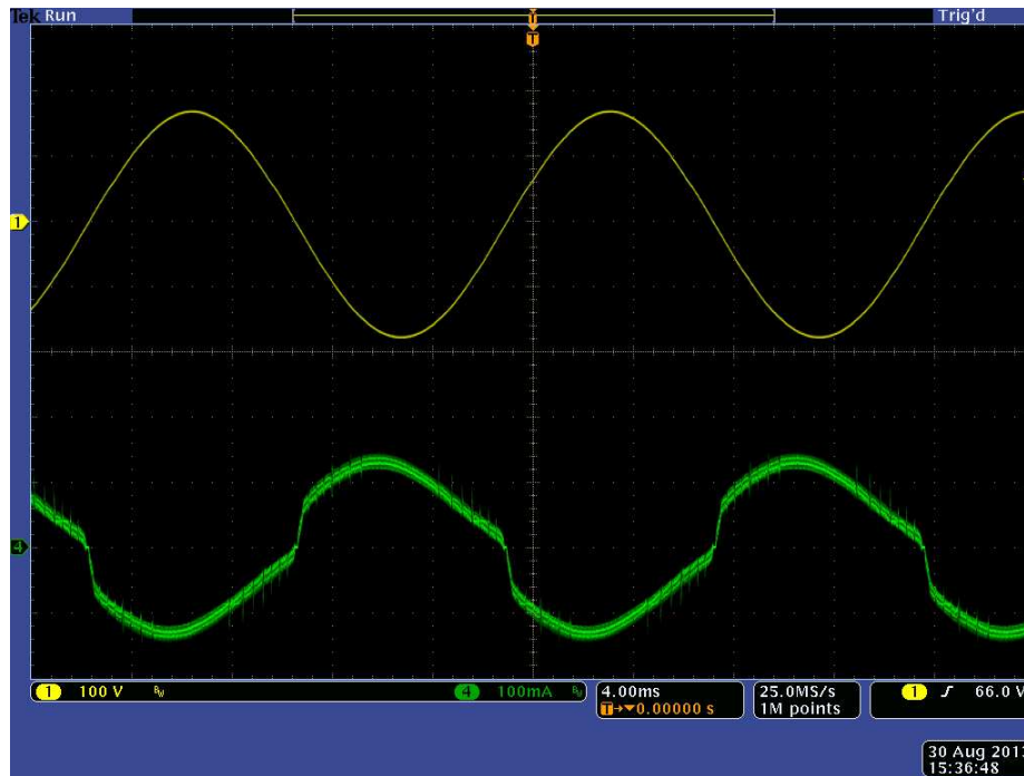
Figure 4. Input Voltage (Top) and Input Current (Bottom)
