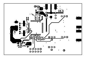
Figure 12. Layer 4 (Bottom Side, View From Bottom)
