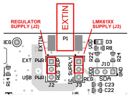
Figure 3. Power Terminals and Jumpers
