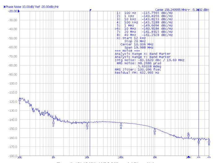
Figure 7. 156.25-MHz LVDS Differential Phase Noise
