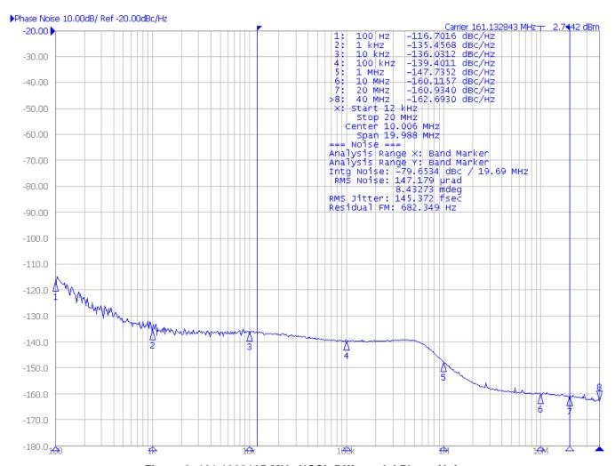
Figure 8. 161.1328125-MHz HCSL Differential Phase Noise
