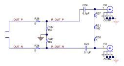
Figure 5. EVM Termination Schematic
