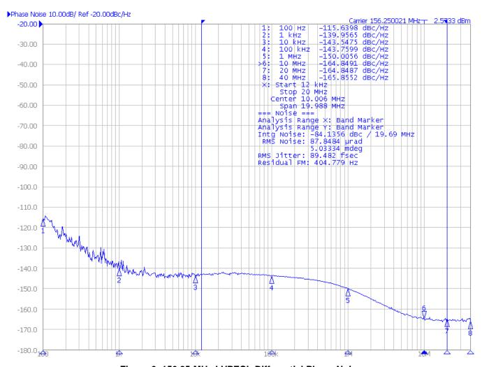
Figure 6. 156.25-MHz LVPECL Differential Phase Noise
