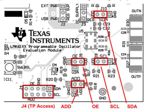
Figure 4. Control Pin Interfaces (Default Jumper Settings Shown)
