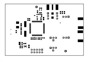
Figure 13. Bottom Solder Mask
