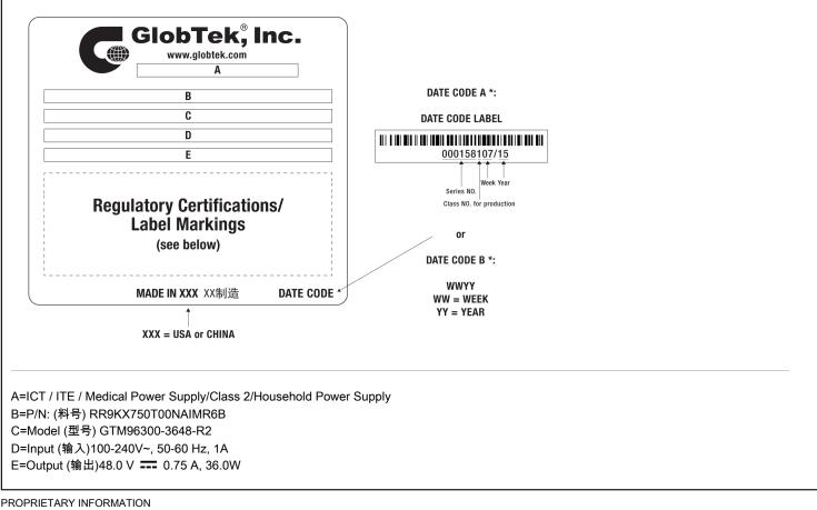
PROPRIETARY OF GLOBTEK, INC. ANY REPRODUCTION, DISCLOSURE OR USE OF THIS DRAWING, IN WHOLE OR IN PART, IS HEREBY PROHIBITED EXCEPT AS SPECIFIED IN WRITING BY GLOBTEK, INC. © GlobTek, Inc. 2016 - 2022 guest /09/17/2022 4:37:09 PM CLONED FROM GS-1046(R)
