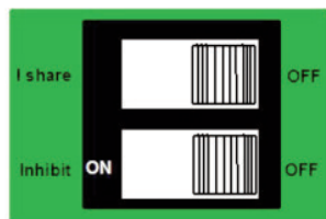
Inhibit OFF/ENABLE ON. Normally OFF
