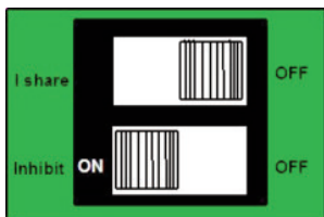
Inhibit ON/ENABLE OFF. Normally ON
