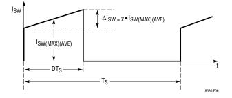
Figure 6. The Switch Current Waveform of the SEPIC Converter
