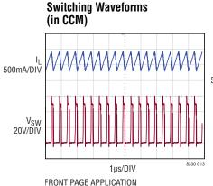
$V_{IN} = 12V$ ,  $V_{OUT} = 48V$ ,  $I_{LOAD} = 135mA$
