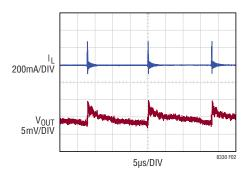
Figure 2. Burst Mode Operation
