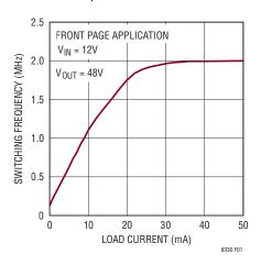
Figure 1. Burst Frequency vs Load Current
