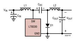
Figure 7. A Simplified Inverting Converter
