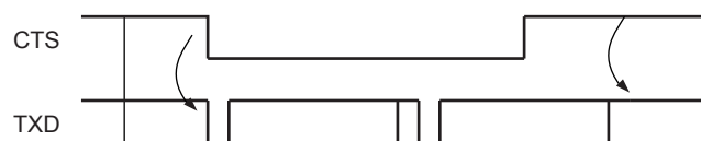
Figure 36-28: Transmitter Behavior when Operating with Hardware Handshaking
